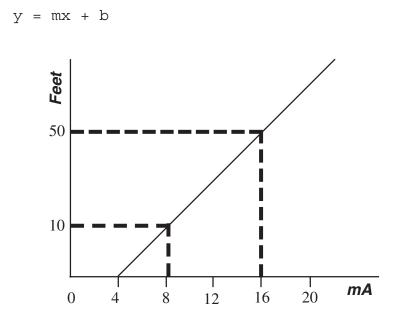
where m is the gain and b is the zero crossing point or Input (ma -> offset. The gain may be calculated from: m=(y2-y1)/x2-x1)
