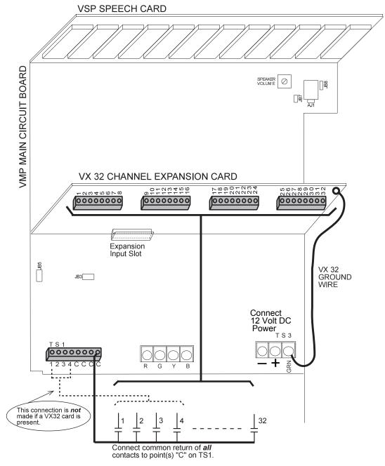
Electrical Connection Diagram For Dry Contact Inputs
