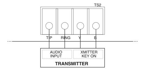
Jumper Wires For RF Link Diagram
