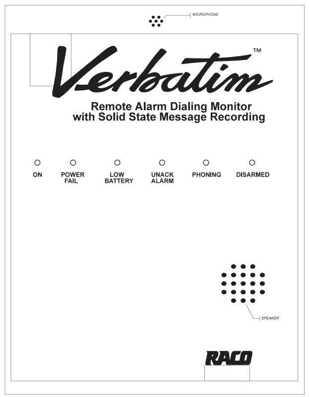
\* A discharged battery may take up to a day to fully charge. \*\* During AC power failure, all illuminated LED's will flash to conserve battery power.
